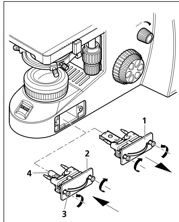
**Fig. 13** Replacing the 6V 30W halogen lamp or the LED illumination module
