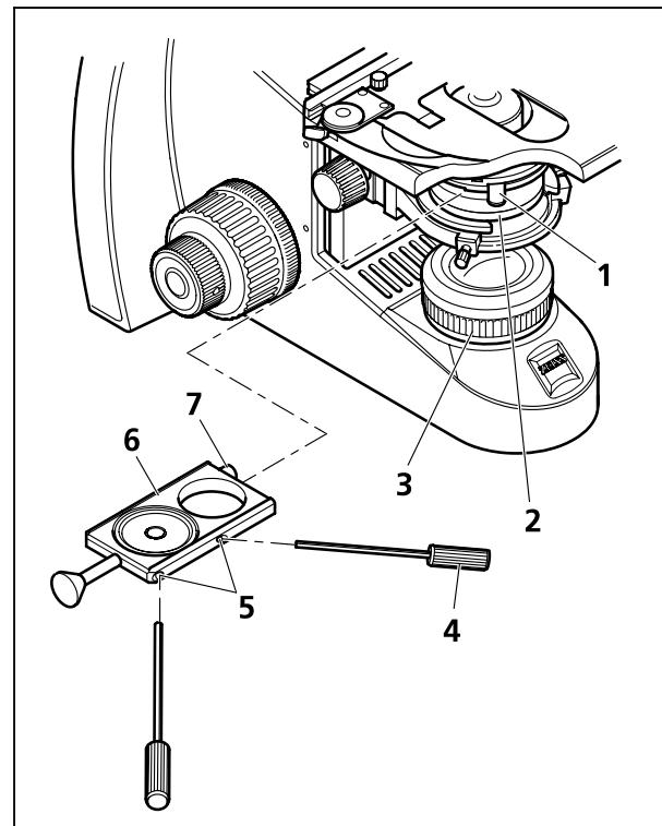
**Fig. 9** Inserting the slider
